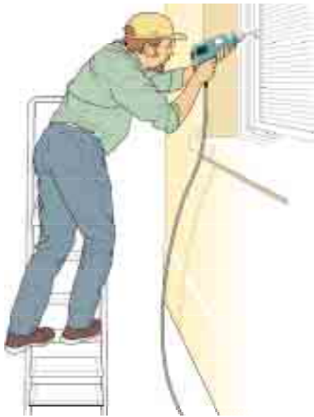
Figure 2a Incorrect - steps side-on to work activity
