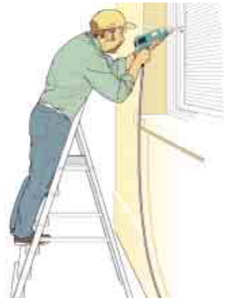
Figure 2b Correct - steps facing work activity
