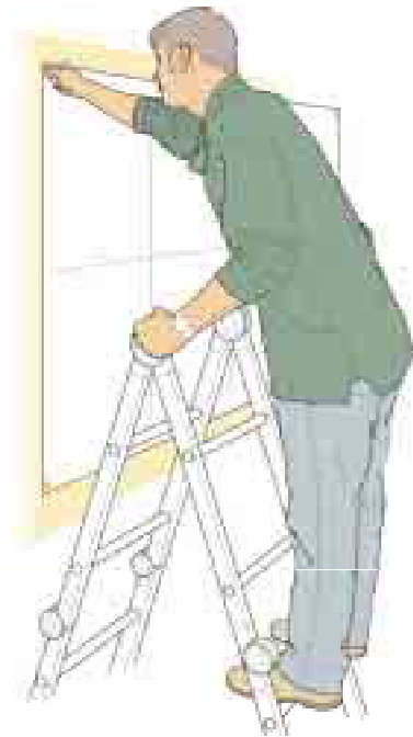
Figure 11 Correct - two clear rungs. Don't work any higher up this type of stepladder
